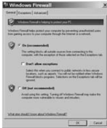
Figure 12-3: The General tab of the Properties window controls the Internet connection firewall.
