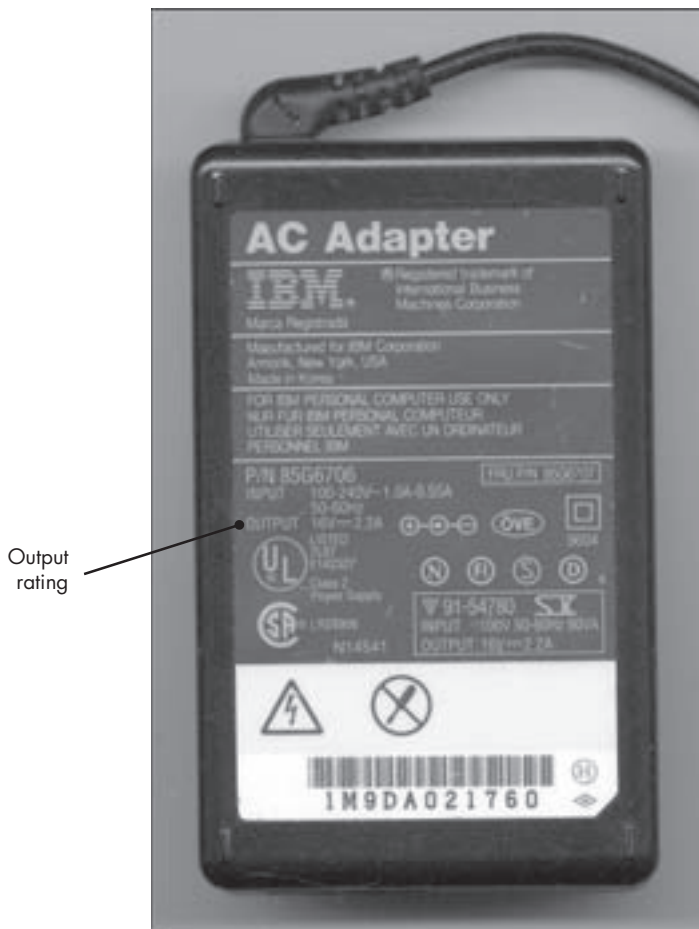
Figure 2-1: This power adapter has an output rating of 2.2 amps at 16V.
