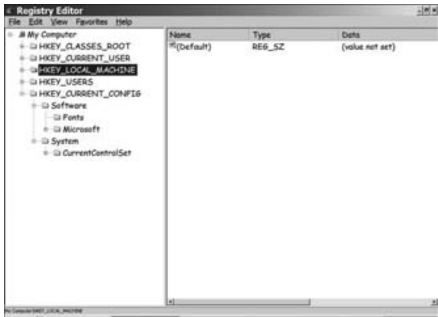
Figure 9-1: Use the Windows Registry Editor to add, change, and remove items from the Registry.
